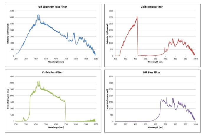
Measured transmission versus wavelength for each filter for an identical PulseForge pulse condition
