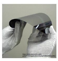
Advanced wafer level packagingthinned wafer debonding
