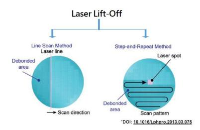
Requires 1000 laser pulses to cover 300 mm wafer\*
