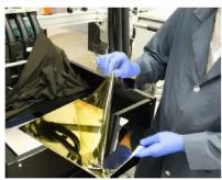
Polymer (≈10 µm) lift-off (360 mm x 465mm – Gen 2)
