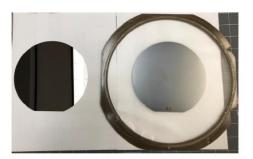
150 mm wafer (60 μm thick) debonded in less than a second
